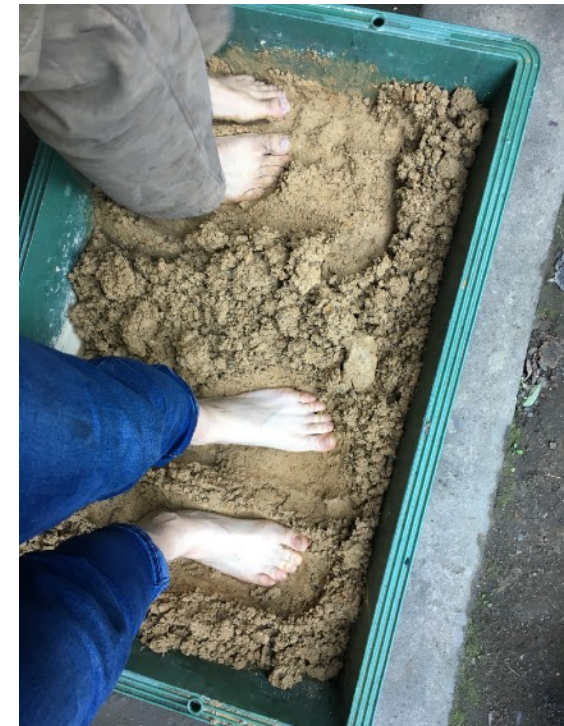
Mixing the clay was done by foot in the Karogane forge.
