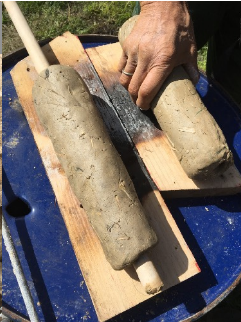
Above - To make the tuyere make a thick sausage of clay wall mix . Use a thin stick to poke a hole and slowly increase its diameter around 3-4cm.
