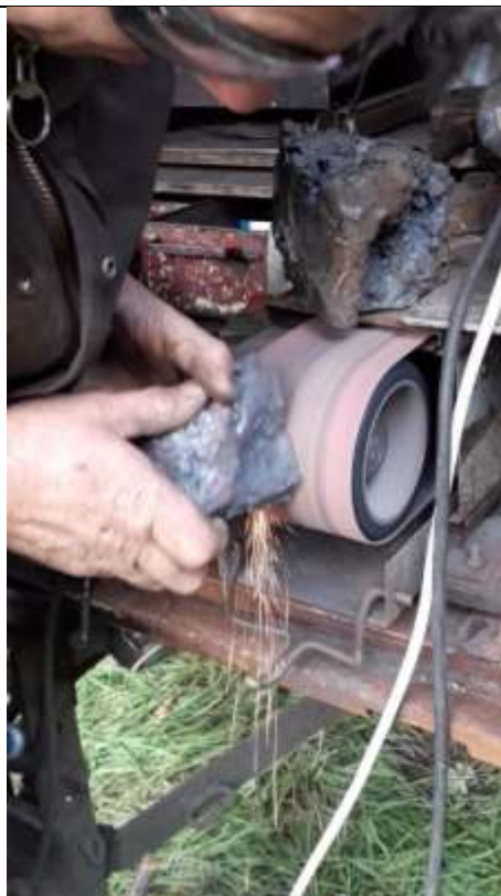
Sparks and also punching confirm that the iron is locally harder, locally softer...
