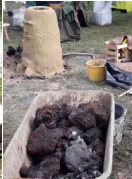
Me, finishing the furnace and the late roast of the other "dark colored" ore from Mountshannon.
