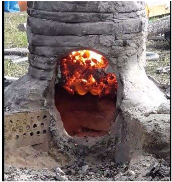
Bloom sticks just beneath the tuyere (top right)
