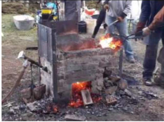
A "Catalan" type furnace:
