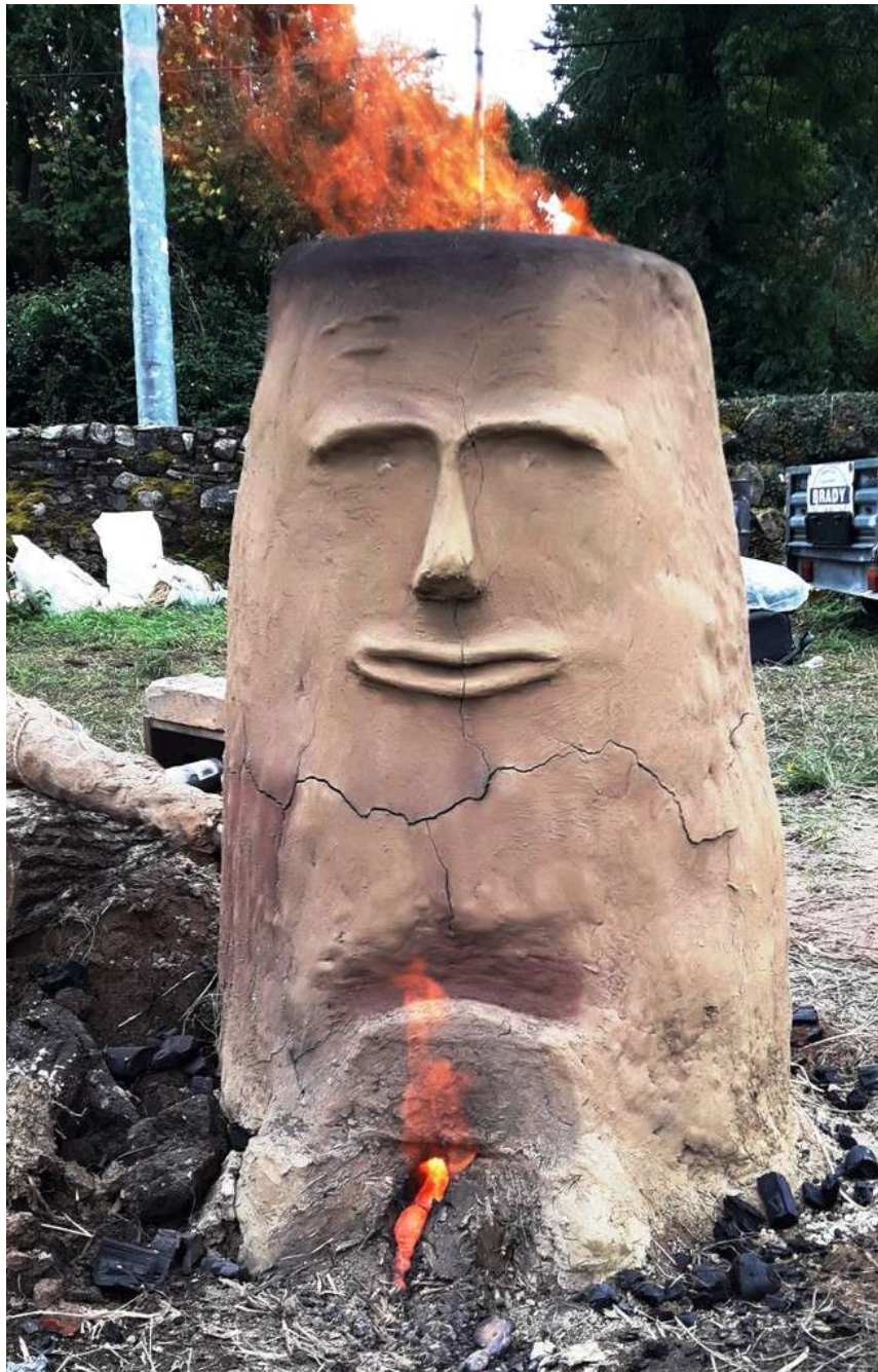
Hard working iron smelting furnace
