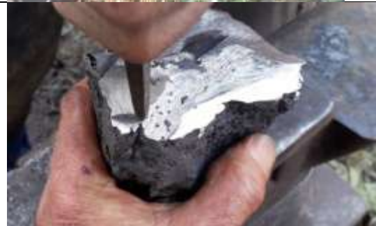
Sparks and also punching confirm that the iron is locally harder, locally softer...
