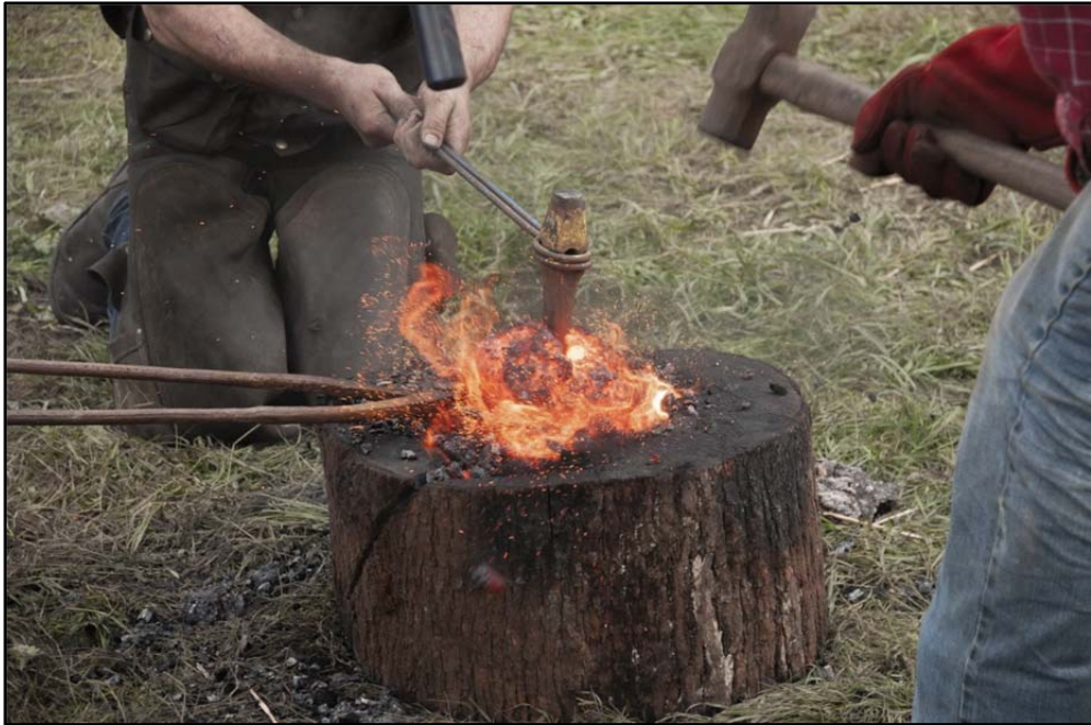
Fig. 3. Splitting the bloom. This activity has two purposes: to test quality of the raw iron and to cut it into easier to work pieces. Furnace Festival 2018 in Woodford, Ireland.
