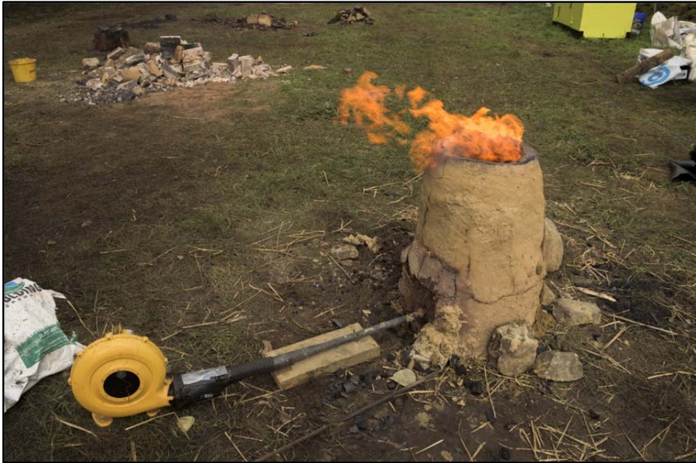
Fig. 1. Small slag-tapping bloomery furnace with artificial air blast. Note other furnaces remains (top left). Furnace Festival 2018 in Woodford, Ireland.
