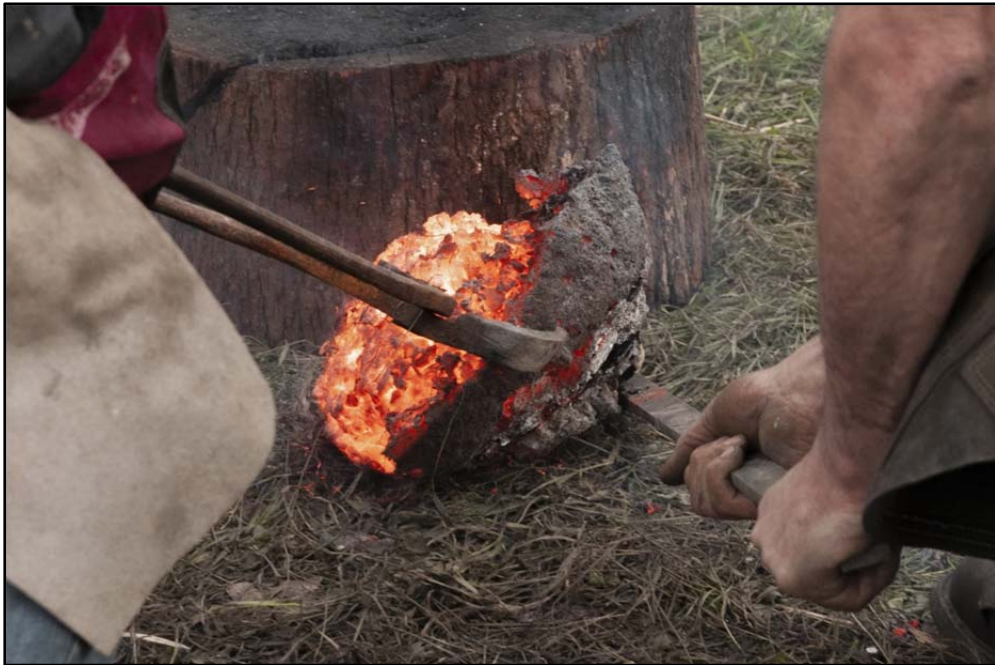
Fig. 2. Bloom (bright) and furnace slag cake (dark). Furnace Festival 2018 in Woodford, Ireland.
