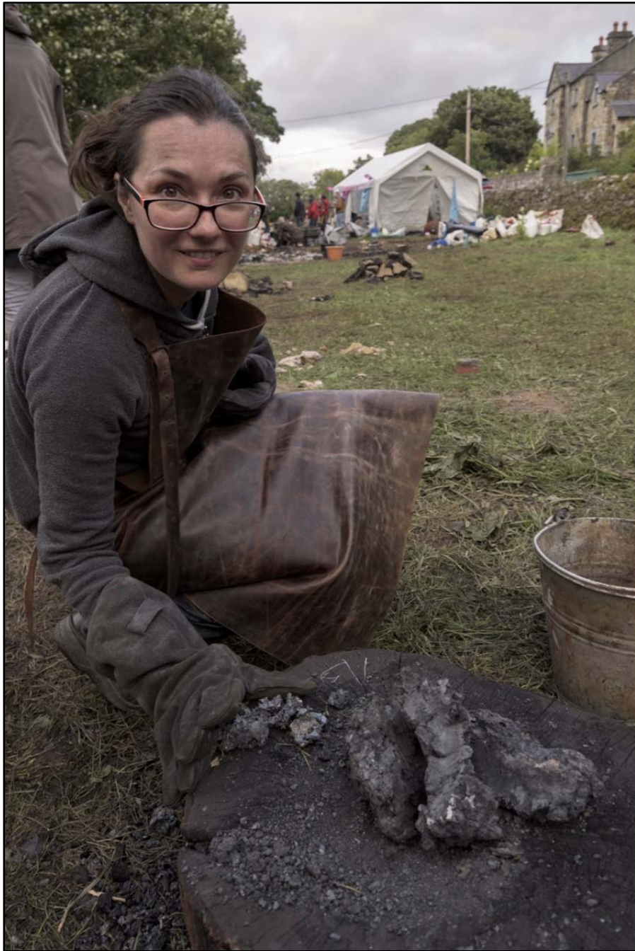
Fig. 4. Daria and her 4.3 kg of iron smelted from 23,4 kg of wet Irish bog ore. The bloom had been compacted and split into three pieces. Furnace Festival 2018 in Woodford, Ireland.
